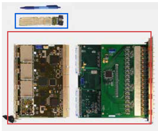
Figure 3: A miniaturized digital receiving module used in dStream coils (blue box) compared with the receiver boards implemented in a MR system (red box)
