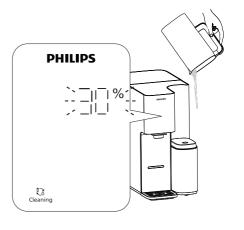
(4) When the " \( \frac{1}{x} \) " indicator light starts blinking, the machine will beep. At this point, remove the tap water tank, empty it, refill it up to the "Max" line, and reinsert it to resume the cleaning.
