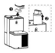
(3) Insert the new filter into the filter holder and rotate it clockwise to the locked " " position, and cover the machine top lid. Put the tap water tank back to the dispenser.
