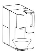
(2) Press and hold the " cold " for 3 seconds, then press the " ( " to begin draining (press again to pause if needed).
