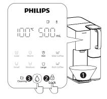
**Caution:** Hot steam may be released during the boiling point adjustment process, which can cause burns. Please keep a safe distance to avoid injury
