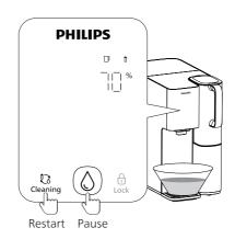
(5) When "100%" flashes, the flushing process is completed.
