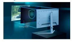
Burn-in is a real concern for users of QD-OLED screens. To increase the lifespan of your display, this monitor has an integrated graphene shield which keeps your display cool. The graphene evenly disperses heat generated by the blue-light emitted from your screen and cools more effectively than graphite. For gamers, this means you can play at the brightness level you prefer with a reduced risk for burn-in, and a display which stays pixel-perfect for longer.
