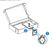
Rotate the bracket to the right and use a screwdriver to loosen the bracket screws.
