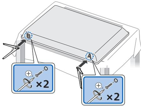
**!** Fasten the stands to the TV with 4 screws (included). While fastening the screws, hold the stand to prevent it from falling.
