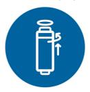
The 5-layer filter cartridge (Philips AUT609R800/00) is tested to keep its performance for at least 6,000 liters of water purification. Recommended to replace after 2 years of usage. A filter lifetime indicator on the smart faucet will remind you when the cartridge is nearing the end of its lifetime and should be replaced.
