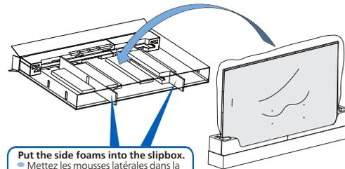
Put the side foams into the slipbox.
