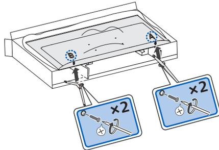
**!** Fasten the stands to the TV with 4 screws (included). While fastening the screws, hold the stand to prevent it from falling. Both stands now be securely fastened.
