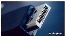
DisplayPort is a digital link from PC to Monitor without any conversion. With higher capabilities than DVI standard, it is fully capable to support up to 15meter cables and 10.8 Gbps/sec data transfer. With this high performance and zero latency, you get the fastest imaging and refresh rates - making DisplayPort the best choice for not only general office or home use, but also for the
