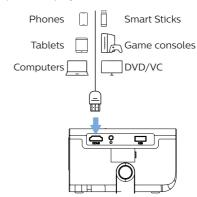
2 If the projector doesn't automatically switch to the correct input source, select **HDMI** from the home screen, or press → on the remote control and select *HDMI*.
