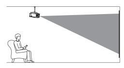
If the projection direction is incorrect, select Settings from the home screen to open the settings menu, go to Display > Projection mode, and press the OK button to select Front Ceiling.
