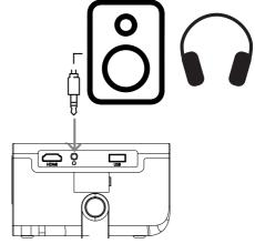
2 After connecting the speakers or headphones, press +/ - on the remote control to adjust the volume to the desired level.
