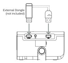
3 If the projector doesn't automatically switch to the correct input source, select **HDMI** from the home screen, or press on the remote control and select *HDMI*.
