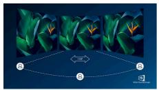
IPS displays use an advanced technology which gives you extra wide viewing angles of 178/178 degree, making it possible to view the display from almost any angle. Unlike standard TN panels, IPS displays gives you remarkably crisp images with vivid colors, making it ideal not only for Photos, movies and web browsing, but also for professional applications which demand color accuracy and consistent brightness at all times.
