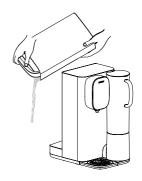
② Fill the tap water tank to the half and add 30g of citric acid. Stir lightly then soak for 2 hours (do not place the tap water tank to the dispenser). Then discard the citric acid solution and clean the entire water tank with tap water.
