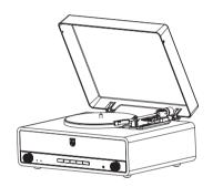
2 Lift up the dust cover vertically from the hinge base.
