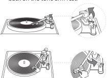
2 Lower the lift lever, and lock the tone arm clip to fix it.
