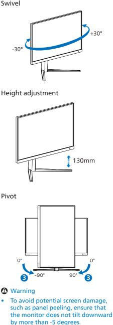
Do not press the screen while adjusting the angle of the monitor. Grasp only the bezel.
