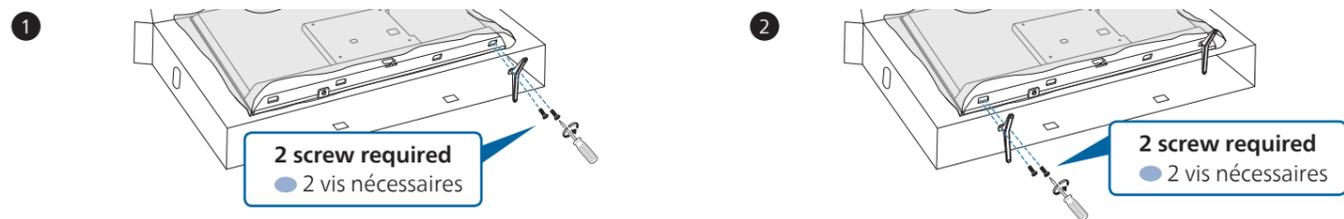
Fasten the stand to the unit with 2 screws each (included).
