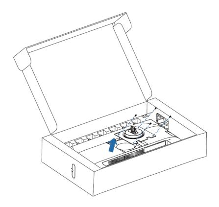
4. Use disassembly tool to open all the latches along the edge of the rear cover, then remove the rear cover.
