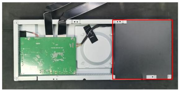
10. Remove tape and screws to get main board and power board.
