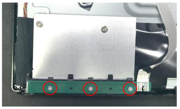
13. Loosen the assembly screws, remove the BKT to get panel.
