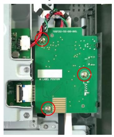
8. Remove tape then disconnect connectors.
