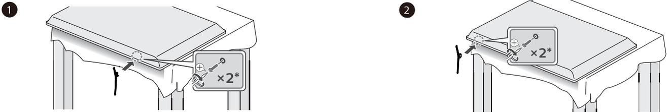
! Prior to attaching each stand, make sure to peel off the protective film where each stand goes in so it will not get stuck between the unit and the stand. Fasten the stand to the unit with 2 screws each (included).
