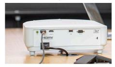
The ProPix 860 features dual HDMI inputs, ensuring seamless integration with legacy systems commonly found in educational institutions and established corporate environments. Also includes a RS232 ports for professional AV control systems, USB connectivity and a 3.5 mm audio output for external sound solutions.
