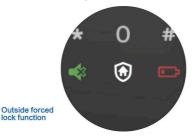
Before leaving home, you can touch the outside forced lock button to enable the function. In this mode, opening the door from inside will trigger an alert. This feature can effectively remind you of security risks and upgrade the level of home
