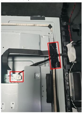
6. Remove the tapes, Mylar and disconnect connectors.
