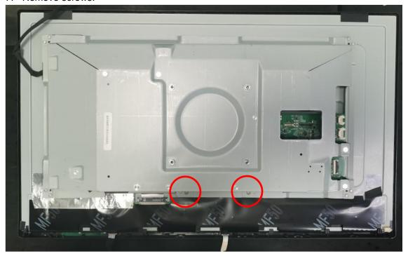
8. Remove the tape then disconnect connector.
