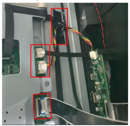
6. Remove the tapes and disconnect connectors.
