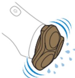
**7** Carefully shake off excess water and let the shaving head holder air-dry completely.
