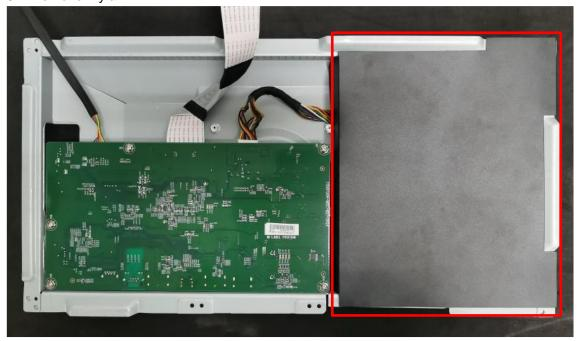
10. Remove screws to get main board and power board.
