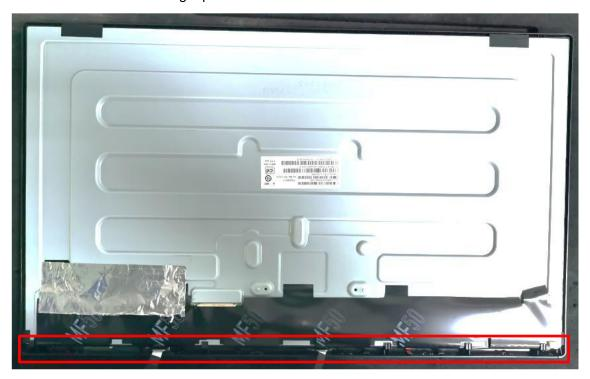
12. Remove screws to get IR board and key board.
