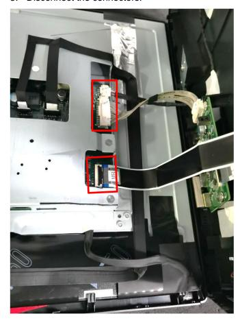
6. Remove the tapes and disconnect connectors.
