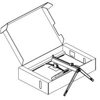
2. While keeping the release button pressed, tilt the stand and slide it out.
