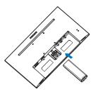
2. Hold the monitor base stand with both hands and firmly insert the base stand into the base column.
