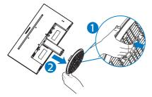
3. Press the release button to detach the base column.
