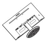
2. Press the release button to detach the base stand away from the base column.
