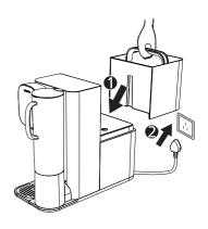
• Please make sure the tap water tank is fully attached to the back panel, otherwise, it will cause improper water filtration or water leakage.
