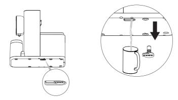
(4) Place a container with a volume of no less than 1 liter under the draining hole. Remove the blue silicone plug to manually drain the cooling tank. Wait until no more water is flowing out, then re-insert the silicone plug tightly.
