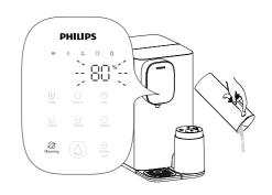
(4) When the " (x " light flashes, you will hear 3 beeps. Empty the water in the tap water tank, refill it with fresh tap water up to the Max line, and place it back.
