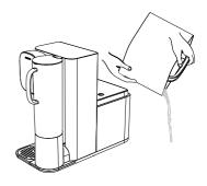
(2) Fill the tap water tank to the half and add 30g of citric acid. Stir lightly then soak for 2 hours (do not place the tap water tank to the dispenser). Then discard the citric acid solution and rinse the entire water tank with tap water.
