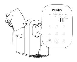
(5) When the progress reaches "90%", and " ( ) " flashes, you will hear 3 beeps. There is no need to empty the water. Place a container with volume no less than 2000ml under the water outlet and press " ( ) ".
