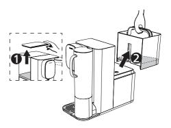
(2) Replenish with tap water to the right level → return the tap water → cover the tap water tank lid
