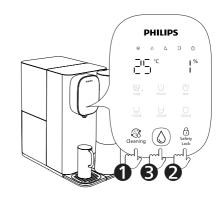
(4) During the cleaning process, press " 🔕 " to pause. Press " 🔕 " again to resume the cleaning process.
