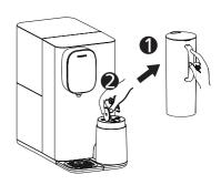
(2) Rotate the used filter cartridge counterclockwise to the unlock " " position and take it out.
