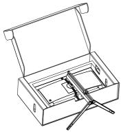
While keeping the release button pressed, tilt the stand and slide it out.
