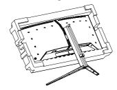
While keeping the release button pressed, tilt the stand and slide it out.
