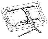
2. While keeping the release button pressed, tilt the stand and slide it out.
