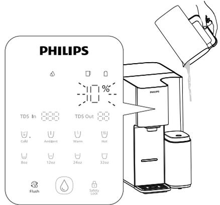
(4) When the "⚠️" light flashes, you will hear 3 beeps. Empty the water in the tap water tank, refill it with fresh tap water up to the Max line, and place it back.
