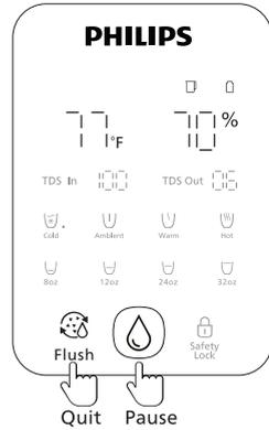
(5) When "100%" flashes, the cleaning process is completed.
