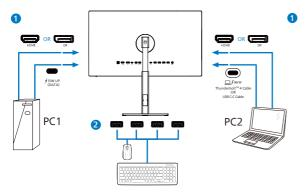
3. Enter to OSD menu. Go to KVM layer and select "USB C" to switch the control of peripherals from one device to another. Simply repeat this step for switching the control system using one set of peripheral.
