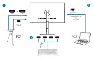
3. Enter to OSD menu. Go to KVM layer and select "Auto", "USB C" or "Thunderbolt" to switch the control of peripherals from one device to another. Simply repeat this step for switching the control system using one set of peripheral.
