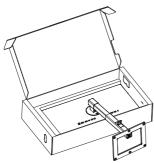
While keeping the release button pressed, tilt the stand and slide it out.
