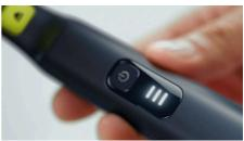
Be sure that your OneBlade is always ready to go by checking the battery indicator. It alerts you while in-use when your battery is low, and indicates charging progress when plugged in.
