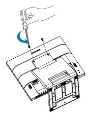
Move the stand into position as shown in picture. Then use a screwdriver to remove the screws, and then detach the stand from the monitor.
