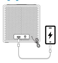
Connect the standard size end of a USB cable (not included) to the USB-type C Port on back of the unit and connect the other end to the charging port on your device.
