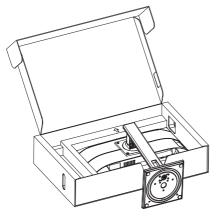
2. Loosen the assembly screws, then detach the neck from the monitor.
