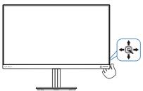
Press to switch power on. 0 Press more than 3 seconds to switch power off. Access the OSD menu. 0 Confirm the OSD adjustment. Adjust the Game Setting. 3 Adjust the OSD menu. Change the signal input source. 4 Adjust the OSD menu. SmartImage Game menu. There are multiple selections: Standard, FPS, Racing, RTS, Movie, LowBlue Mode, EasyRead, Economy, Game 1, Game2. When the monitor receives 6 HDR signal, SmartImage will show the HDR menu. There are multiple selections in
