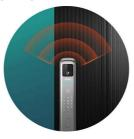
The DDL702-MVP-17HWS features a wide-angle camera and four low-power infrared lights, offering both day and night vision modes. In low light, the infrared lights automatically activate, transitioning to night vision. This ensures clear facial recognition within a 2-meter range, even in dimly lit environments near the lock.
