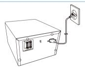
Connect the power cable to the wall socket.
