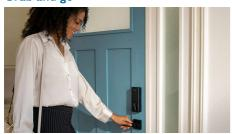
The built-in proximity sensor detects your hand reaching toward the indoor knob or lever and sends unlock signals to the lock. The deadbolt will automatically unlock as you reach toward the knob, allowing you to leave with ease and not have to physically unlock the deadbolt yourself. This feature is disabled by default.
