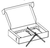
While keeping the release button pressed, tilt the stand and slide it out.
