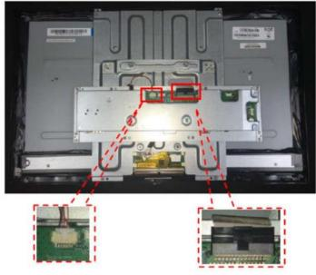
5. Remove the screws to remove the mainframe from
