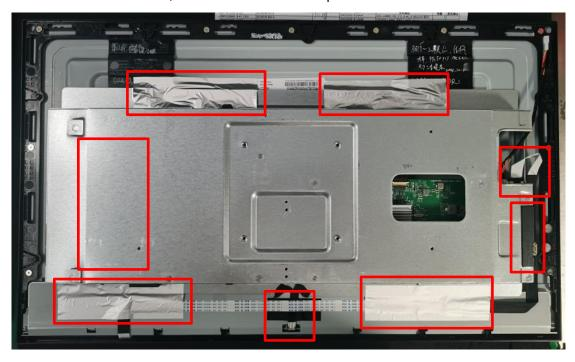
6. Throw the main frame from one side, take off the tape and disconnect the connectors. Then remove the main frame.
