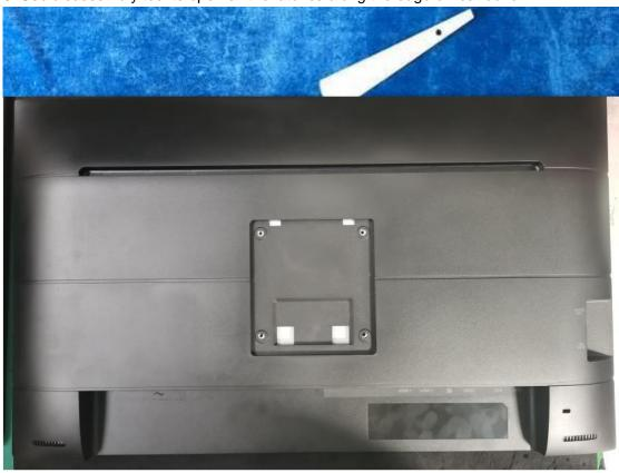
4. Throw the rear cover from one side, then take off the tape and disconnect the connector.
