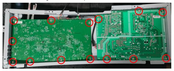
10. Remove screws to get middle frame and panel.
