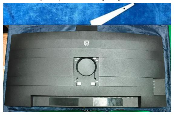
4. Take off the tapes and connector then remove the rear cover.
