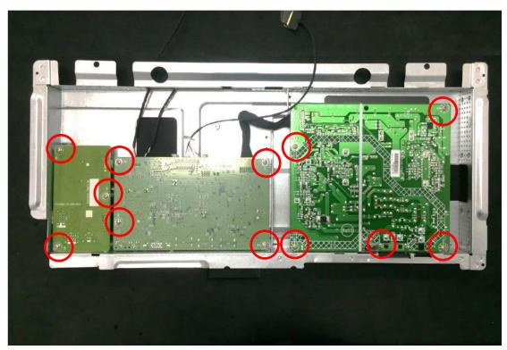
8. Remove screws to get middle frame and panel.
