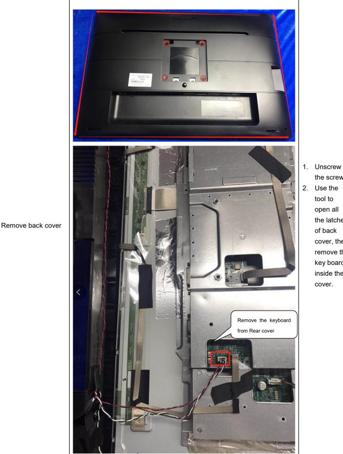
the screws Use the tool to open all the latches of back cover, then remove the key board inside the cover.
