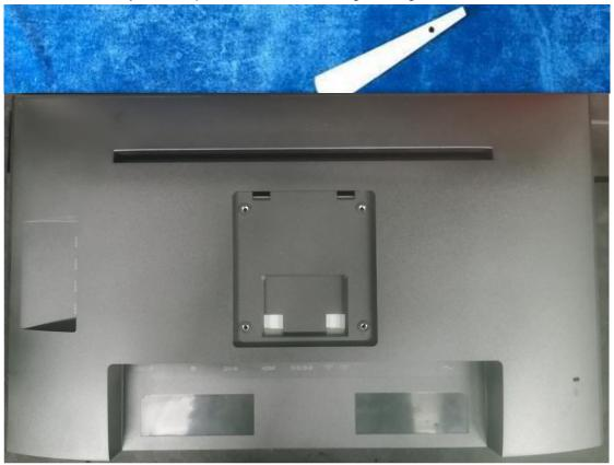
4. Throw the rear cover from one side, then take off the tapes and disconnect the connector.
