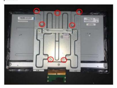
6. Remove the screws to remove the board.
