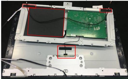
3) Remove the screws to remove the middle frame and the panel.
