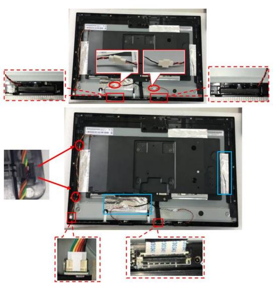
4. Remove the table and connector cable and Mylar.
