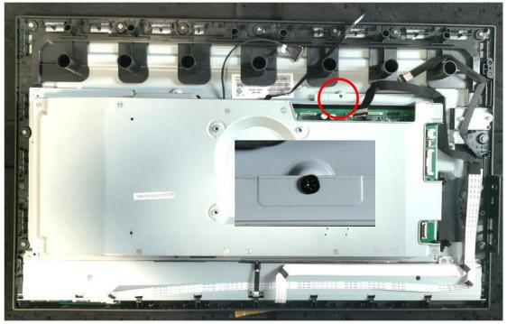
8. Throw the main frame from one side, take off the tape and disconnect the connectors. Then remove the main frame.
