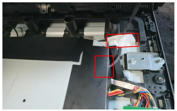
5. Remove the rear cover, then take off all of the tapes and disconnect the connectors.
